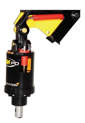
Integrated into the hitch & drive hood, Digga's swing control uses grease filled cylinders to reduce the forward /back and side to side movements of your auger drive and auger. It is fully independent of your hydraulic system requiring no additional hosing.
